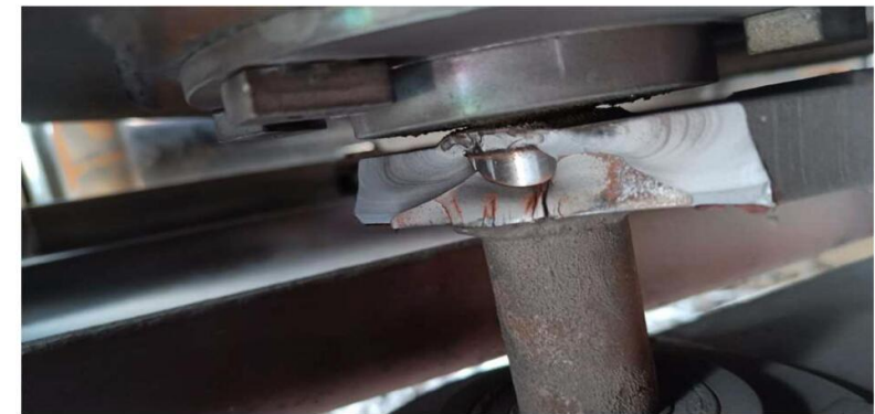
Fig 3- Failures of bell crank lever near the pivot pin
