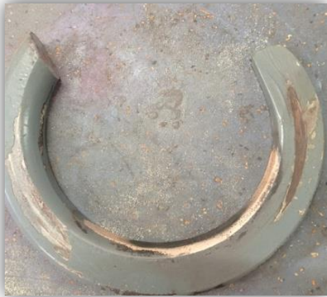
1 st Case Rly- VSKP Location: Top Rubbing mark of length 140 mm noticed on inner bottom side of the end coil and outer surface of the first active coil indicating mutual rubbing of these two coils in service.
