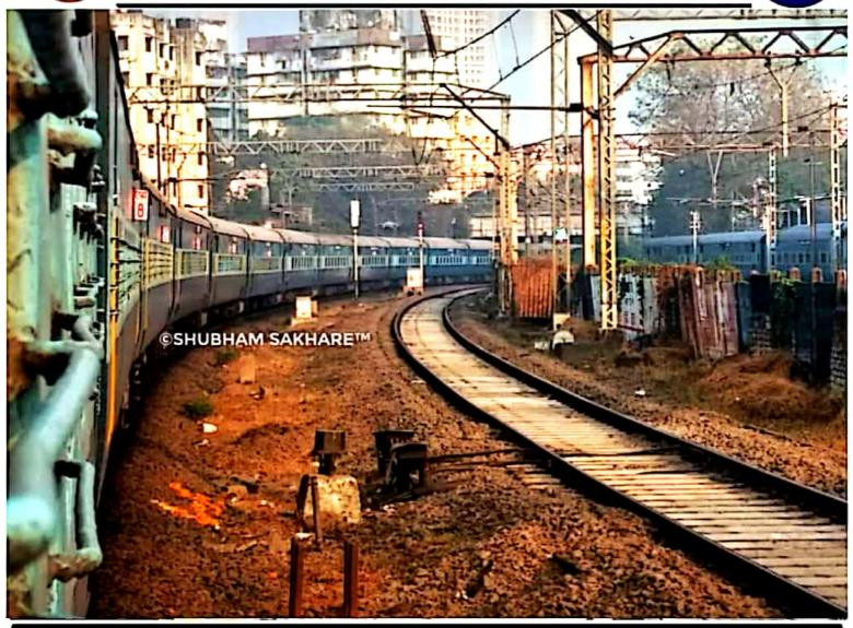
The minimum curve radius selected for Indian Railways broad gauge tracks is 175 m(574 ft). It is the shortest allowable design radius for the centerline of railway tracks under a particular set of conditions.
