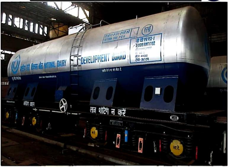
Indian Railways have developed a new Rail Milk Tank van which has carrying capacity of 44,660 litres of milk, which is almost 12 % more than the earlier van. It has been indigenously manufactured to run at speeds of up to 110 kmph and will facilitate safe, economic as well as quick transportation of milk.
