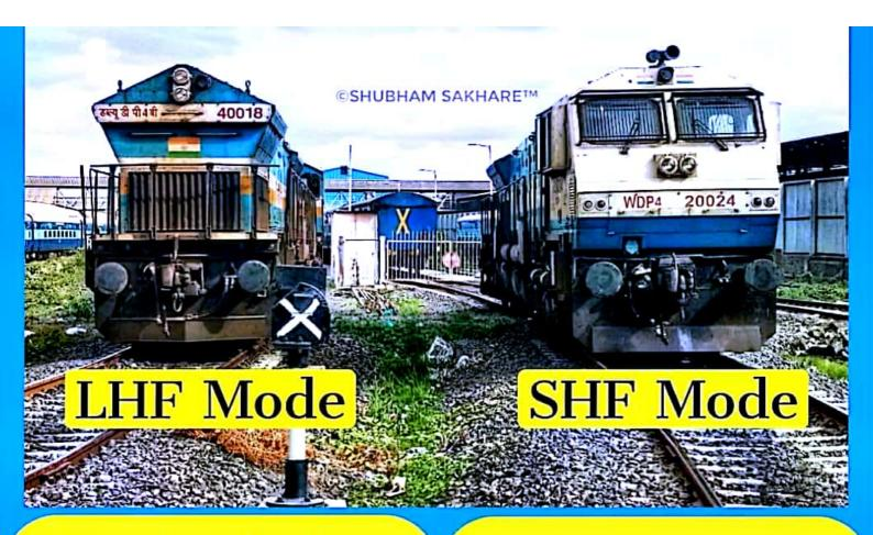
LHF mode is the driving style where the locomotive is driven with the driving cab behind the longer Hood length of the loco body technically reverse operating position.
